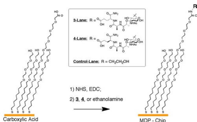
**Figure 2.** Synthesis of the MDP chip. A mixed SAM consisting of 1 mol % hexa(ethylene glycol)carboxylic acid [(EG)<sub>6</sub>CO<sub>2</sub>H]-terminated thiol in tri(ethylene glycol) [(EG)<sub>3</sub>OH]-terminated thiol was prepared. The carboxylic acid groups were then activated with NHS and EDC to form NHS esters. Displacement of NHS esters with the amino groups of MDPs formed amide bonds. Excess NHS esters were deactivated with ethanolamine.
